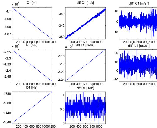
Fig. 6. Raw code measurement, carrier phase measurement, and Doppler shift - simple analysis of signal without failure.
