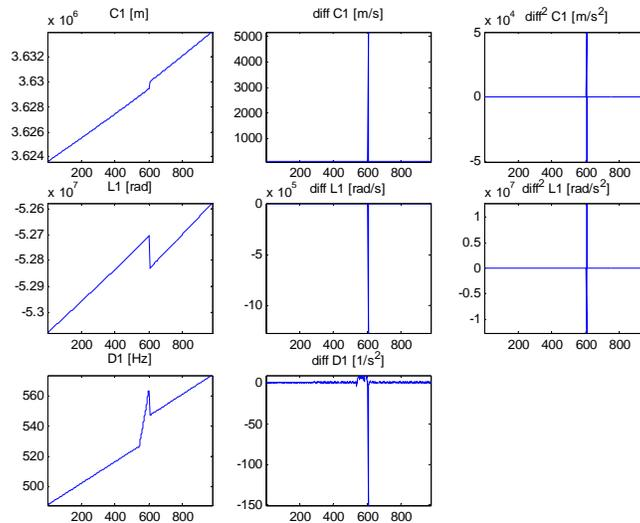
Fig. 7. Raw code measurement, carrier phase measurement, and doppler shift - simple analysis of signal with discontinuity.
