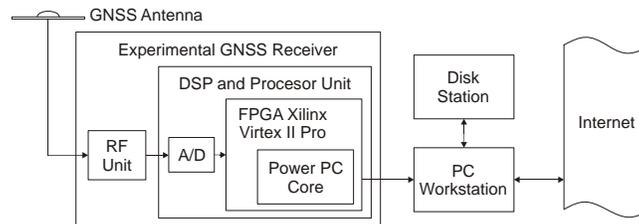
Fig. 1. GNSS monitoring station architecture.
