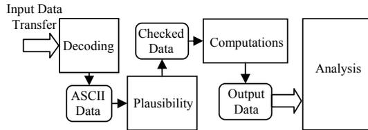
Fig. 2. PEGASUS data processing structure [3].
