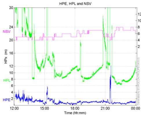
Fig. 3. Horizontal position error, horizontal protection limit (HPL), and number of satellites in view (NSV).
