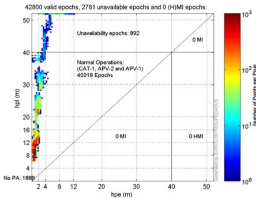
Fig. 4. Horizontal Stanford plot.
